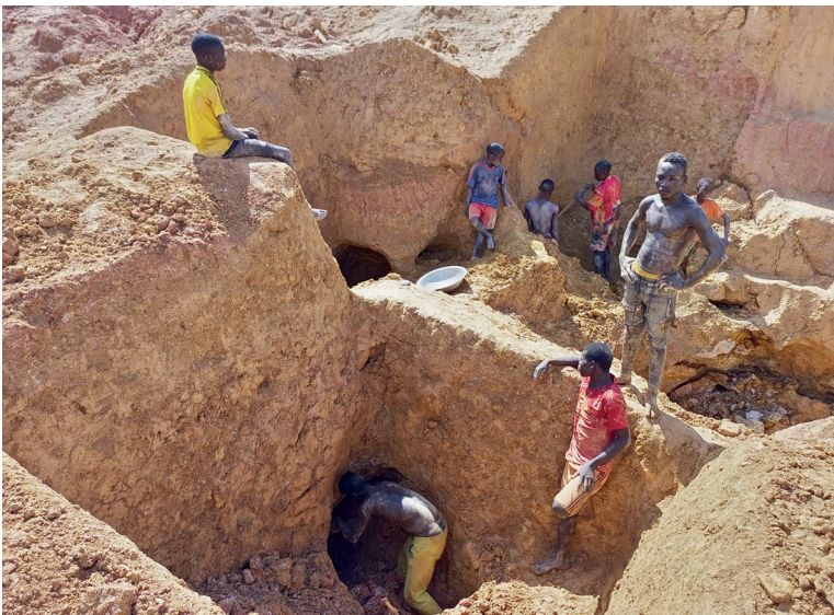
Figure 3. Different steps in the artisanal gold mining process: Open pits (A); entrance into a tunnel (B);
