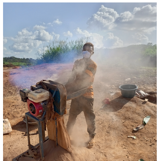
Figure 3. Different steps in the artisanal gold mining process: crushing of hard rock (C); grinding (D);
