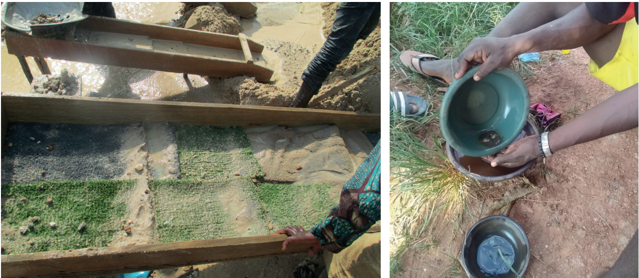
Figure 3. Different steps in the artisanal gold mining process: Sluicing (E); amalgamating (F).
