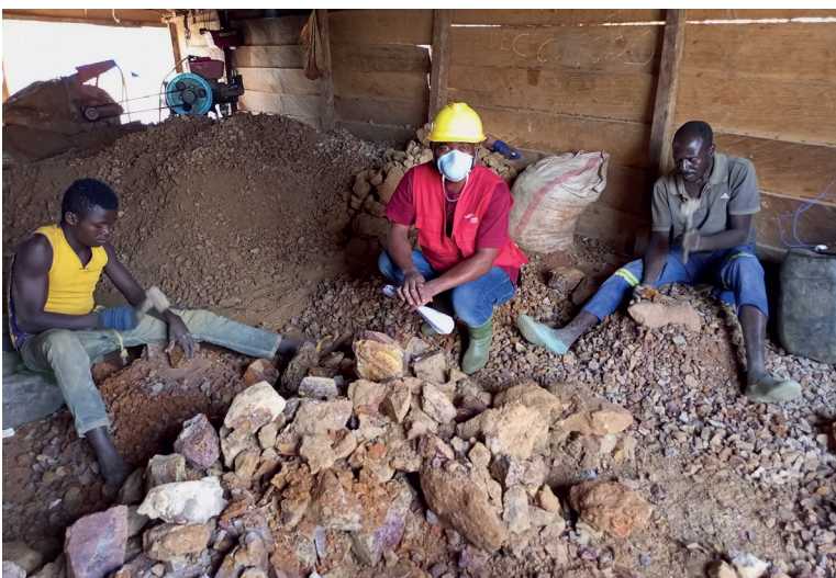
Figure 3. Different steps in the artisanal gold mining process: crushing of hard rock (C); grinding (D);
