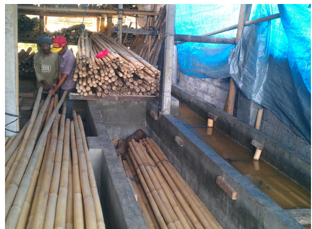
Photo 5: Soaking bamboo in water or leaching Photo source: bellobamboo.com
