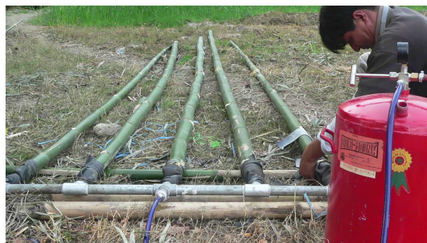
Photo 8: Bamboo boucherie treatment Photo source: INBAR
